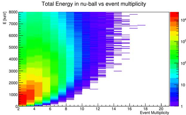
Fig. 3. Multiplicity *versus* total deposited energy in  $\nu$ -ball spectrometer during activation of the  $^{232}\text{Th}$  target.
