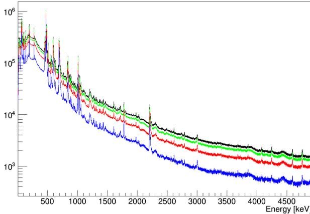
Fig. 6. (Color online) Delayed gamma spectra during the measurement of spectroscopy above the shape isomer in  $^{238}\text{U}$  (from 100 ns to 300 ns after beam pulse) with prompt gamma multiplicity equal to or less than 1 and delay gamma multiplicity: equal or less than 1 (bottom/blue line), equal or less than 2 (second from the bottom/red line), equal or less than 3 (second from the top/green line) and equal or less than 4 (top/black line).
