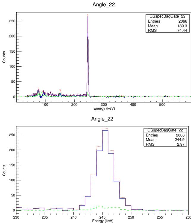
Fig. 4. (Colour on-line) Gated spectra from the bin 22 angular correlation matrix that corresponds to  $\theta = 47.4^\circ$ . (top) A spectrum gated on the 151 keV  $\gamma$  ray (dotted red line); a background spectrum gated on a region next to the 151 keV peak (dashed green line); and a background-subtracted spectrum, made as a difference between the two former spectra (solid blue line). (bottom) The same as upper figure but zoomed around the 245 keV peak.
