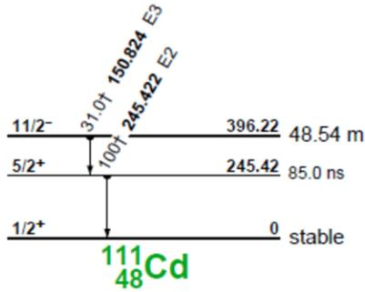
Fig. 2. Partial level scheme of  $^{111}\text{Cd}$  [6].
