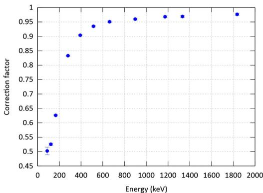
Fig. 2. Self-absorption correction factors for tungsten.
