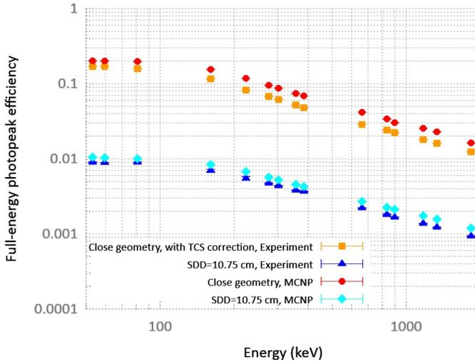
Fig. 1. Measured and calculated FEPE at two source-to-detector distances for point-like sources: Am-241, Ba-133, Cs-137, Mn-54, Co-60 and Y-88.
