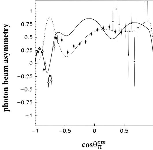
Fig. 1. Photon beam asymmetries measured by BGOegg (closed circles), LEPS (open crosses), and Daresbury (closed stars) at  $2200 < E_\gamma < 2300$  MeV. Solid and dashed curves represent partial wave analysis calculations by SAID and Bonn-Gatchina groups, respectively.
