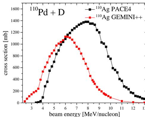
Fig. 3. Total cross sections for  $^{110}\text{Ag}$  production in  $^{110}\text{Pd} + \text{D}$  fusion–evaporation reactions obtained using the PACE4 and GEMINI++ codes.
