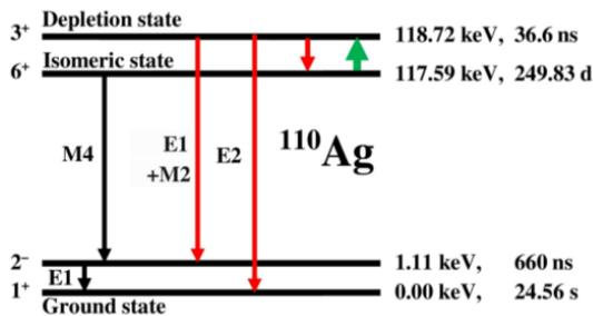
Fig. 1. Partial level scheme for  $^{110}\text{Ag}$  nucleus (not to scale). Data are from [11].
