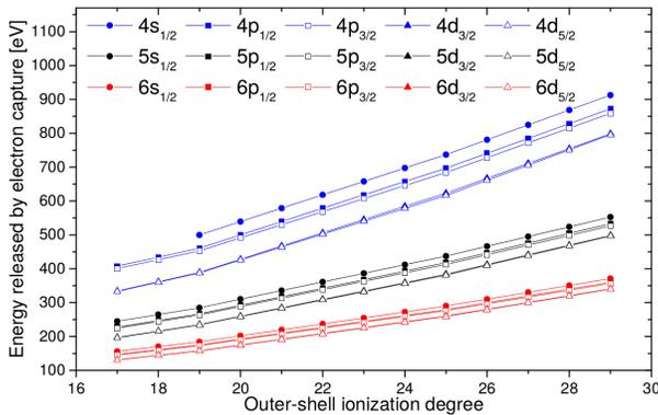
Fig. 4. Dependence of the energy released by electron capture into  $N$  ( $n = 4$ ),  $O$  ( $n = 5$ ) and  $P$  ( $n = 6$ ) subshells of  $^{110m}\text{Ag}$  isomer on the outer-shell ionization degree.
