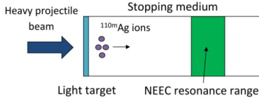
Fig. 2. The NEEC process experimental observation scheme for the  $^{110m}\text{Ag}$  isomer (concept adapted from [12]).
