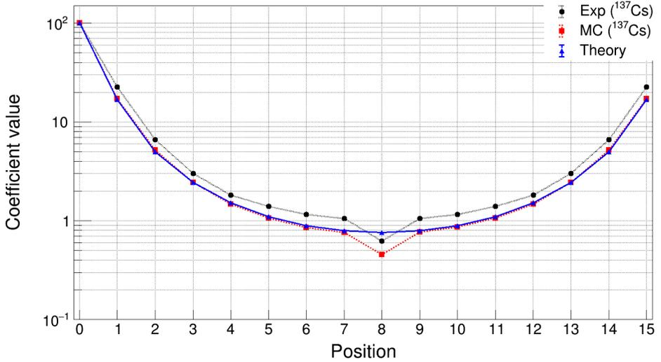
Fig. 4. The influence of other sources to the strength of principal signal for a rotating wheel with 16 sources, normalized to 100 at 0 position, is obtained from the experiment, the theoretical model  $f_{16}$  (Eq. (14)), and Geant simulations.
