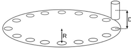
Fig. 1. Schematic view of the experimental apparatus composed of a rotating disk (samples placed at radius  $R$ ) and  $\gamma$ -radiation detector placed at (effective) distance  $D$  from the surface of the disk.
