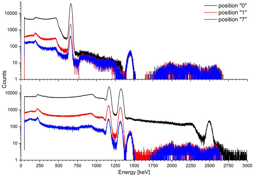
Fig. 3. Energy spectra measured for three positions of the source: position 0 just above the detector, position 2 corresponding to the rotation of the disk by  $45^\circ$ , position 7 corresponding to the rotation of the disk by  $157.5^\circ$ . The top (bottom) panel is for <sup>137</sup>Cs (<sup>60</sup>Co) source.
