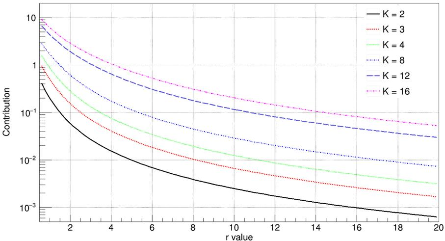
Fig. 2. The relative excess contribution of neighboring samples with respect to that close to the detector, for selected numbers of samples on the rotating disk ( $K = 2, 3, 4, 6, 8, 12, 16$ ). The line for  $K_n$  is above  $K_m$  for  $n > m$ , as the contribution is additive.
