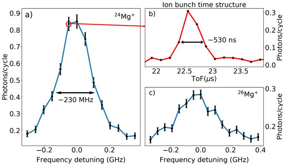
Fig. 2. (a) D2-line resonance of  $^{24}\text{Mg}^+$  ions averaged over 500 measurement cycles per frequency step. (b) Fluorescence signal over time of flight (ToF) for the resonance frequency of  $^{24}\text{Mg}^+$  ions. (c) Resonance of  $^{26}\text{Mg}^+$  ions averaged over 2 000 measurement cycles.
