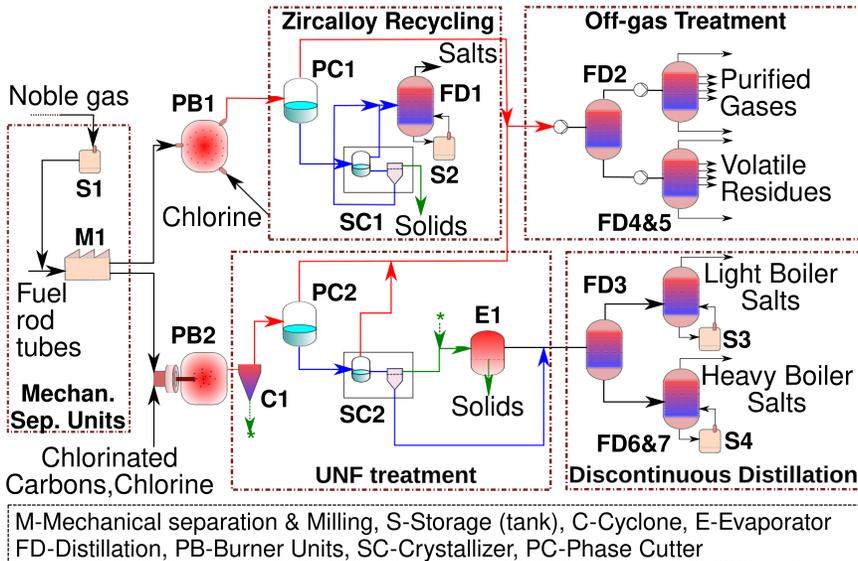
Fig. 2. Simplified flow chart of the Pyroprocessing Unit (PPU).
