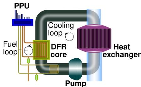
Fig. 1. The DFR fuel and cooling loops for a 1500 MWe DFR.
