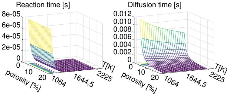
Fig. 4. Timescale: Simulation results for the chlorination of UNF on basis of uranium tetrachloride.
