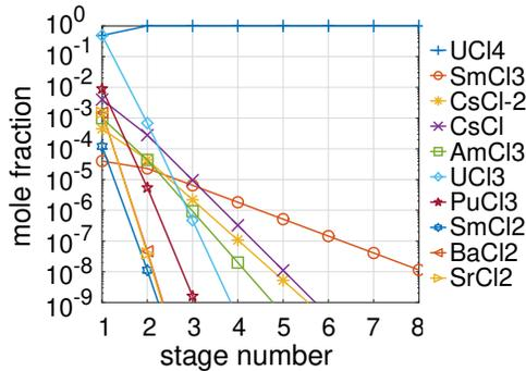
Fig. 3. Continuous fractionated distillation column results.
