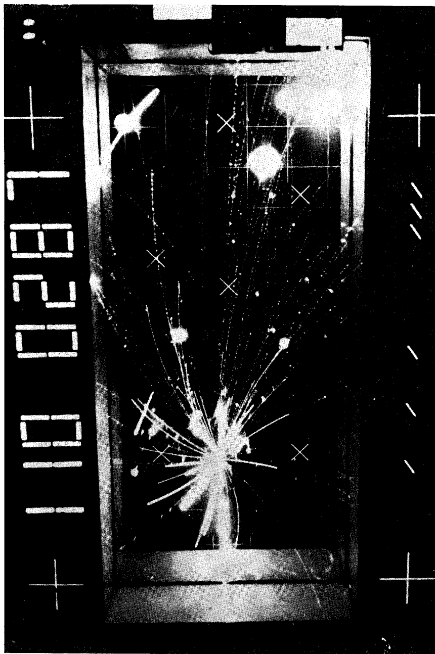
Fig. 21. 1.8 GeV/nucleon ^{40}\text{Ar} projectile interacting with a thin \text{Pb}_3\text{O}_4 target inside LBL streamer chamber. Positive particles bend down in magnetic field of chamber, and negative particles bend up
