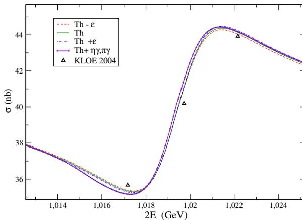
Fig. 1. Muon pair cross section. The comparison between theory and experiment as described in text.
