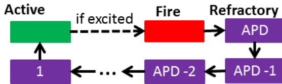
Fig. 2. An excited automaton in the active state becomes firing. Then it moves to the refractory state and spends there APD steps, after which it returns to its original state of being active.
