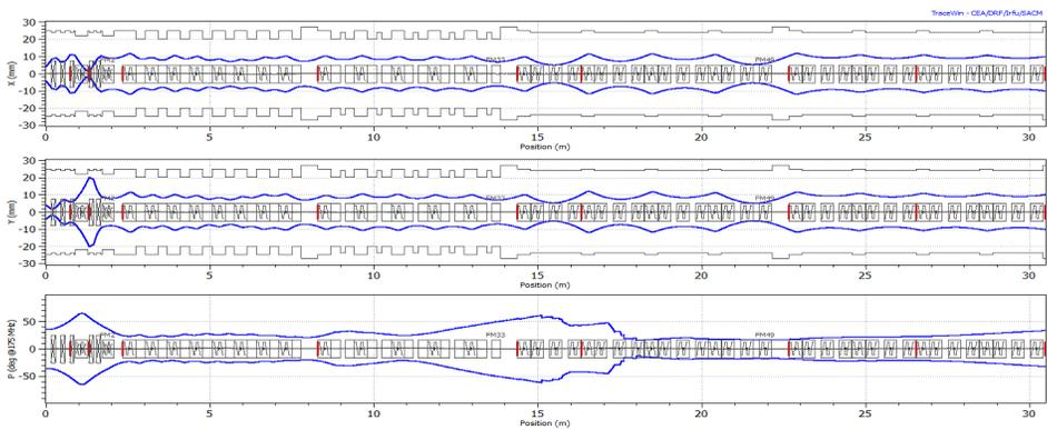
Fig. 4. Envelopes of the deuteron beam. Upper: X-direction; middle: Y-direction; bottom: phase envelope.
