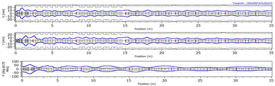
Fig. 6. Envelopes of the deuteron beam. Upper: *X*-direction; middle: *Y*-direction; bottom: phase envelope.
