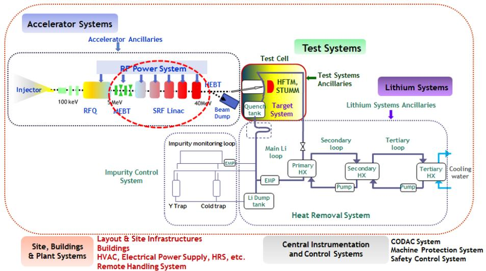
Fig. 1. DEMO-oriented neutron source. A part interesting for us is marked with the dashed line. Courtesy of Prof. W. Królas.
