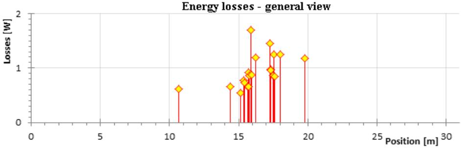
Fig. 2. Localisation of beam energy losses for the best variant calculated with TraceWin.
