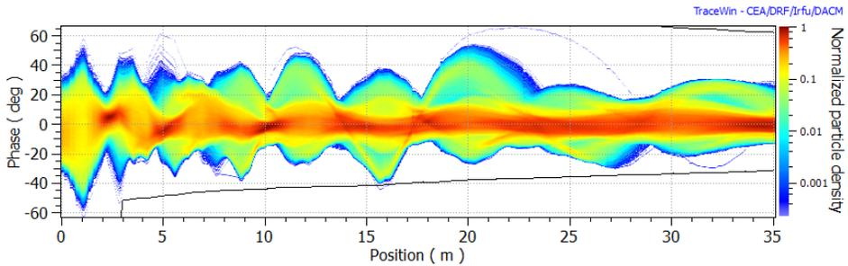
Fig. 5. Phase density of the deuteron beam.
