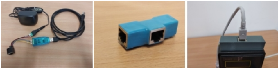
Fig. 4. The parts of the dosimetry system. Left: the way of connecting power supply and RS-485 bus signals from the USB-RS485 converter. Center: T-branching signals on the RS-485 bus. Right: new EKO-C connector.
