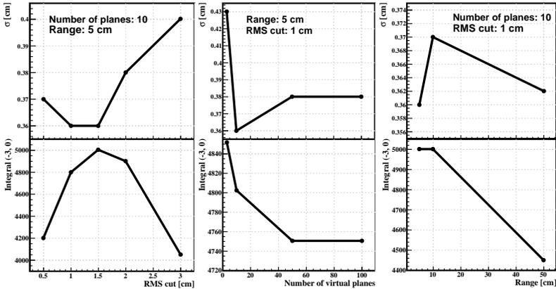
Fig. 3. Dependence of vertex quality on tuning parameters.
