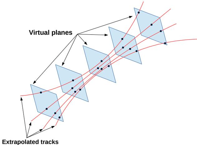
Fig. 1. Graphical explanation of vertex finder algorithm.
