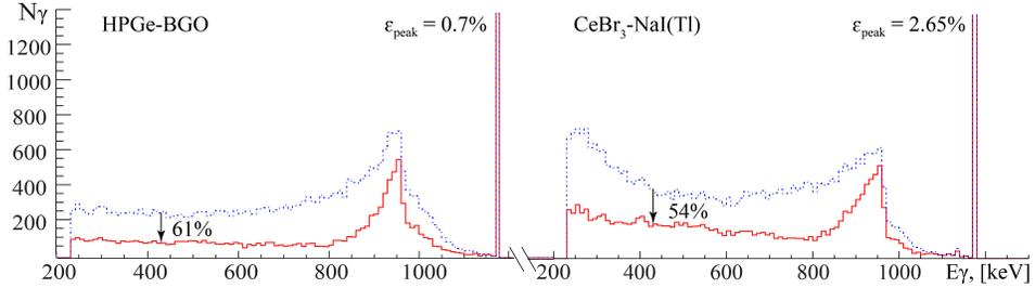
Fig. 3. The Geant4 calculated energy spectra of the HPGe-BGO detector (left) and central CeBr<sub>3</sub>-NaI(Tl) detector of the cluster (right). The dashed lines are inclusive spectra, the solid lines are Compton suppressed spectra.
