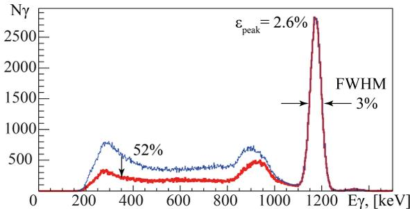
Fig. 4. The energy spectrum of CeBr<sub>3</sub>-NaI(Tl) central detector of the cluster measured by the tagged  $\gamma$ -rays technique.
