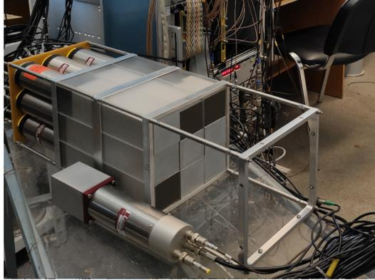
Fig. 1. The cluster of  $9 \times \text{CeBr}_3\text{-NaI(Tl)}$  phoswich detectors manufactured by Scionix Holand B.V. [3].
