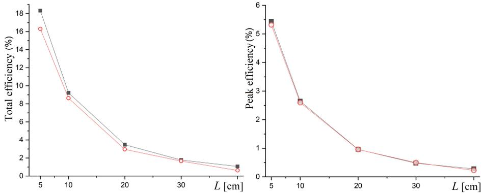
Fig. 6. Total efficiency and peak efficiency as a function of distance to  $\gamma$ -source  $^{60}\text{Co}$ . The measurements for target  $\gamma$ -quanta with  $E\gamma = 1173$  keV. Squares — calculated results, circles — measured results.
