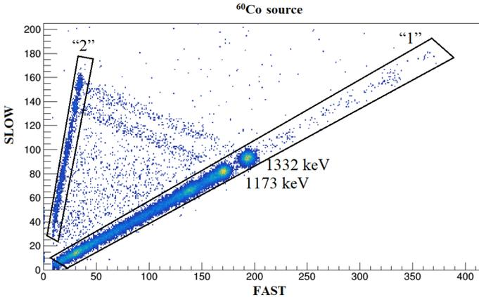
Fig. 5. 2D-matrix of MDPP-16 pulse processor unit (running in QDC mode). On the X-axis is the FAST with integration time 25 ns and Y-axis is the SLOW with an integration time 380 ns.
