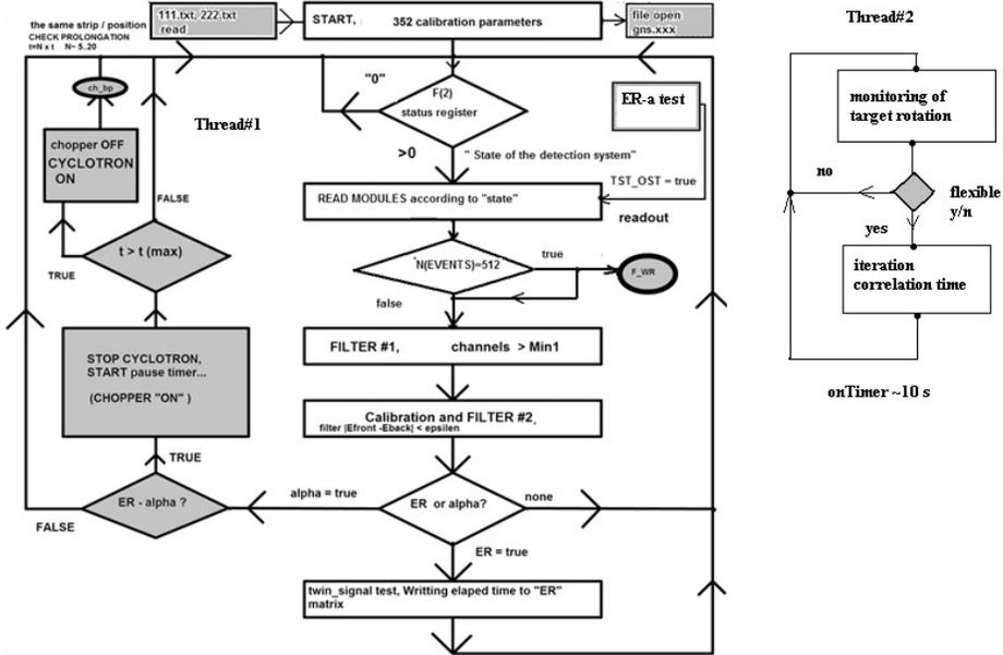
Fig. 3. Flowchart of YDA program main process.
