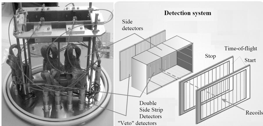
Fig. 1. Schematic view of the detection module. DSSSD detector, side detectors and two multiwire low pressure proportional chambers are shown.
