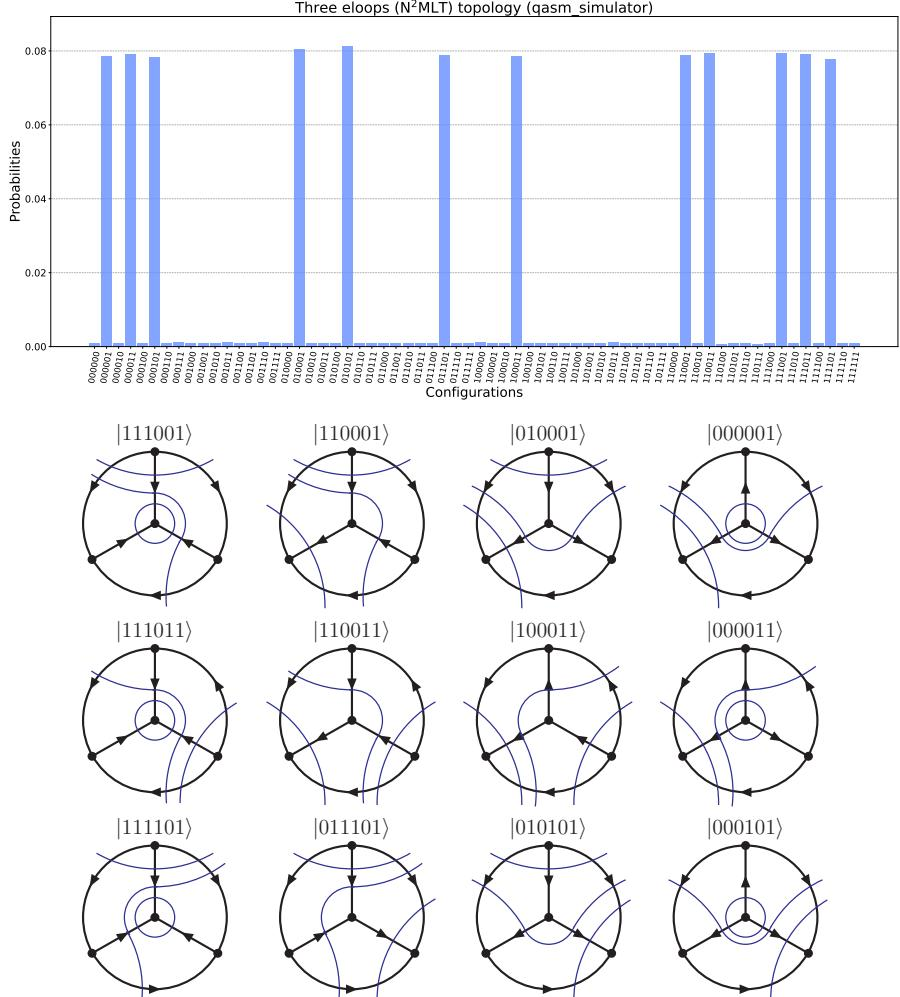
Fig. 5. Probability distribution output of the quantum circuit (top) and the associated entangled causal thresholds (bottom) for the N<sup>2</sup>MLT topology with one edge by set.
