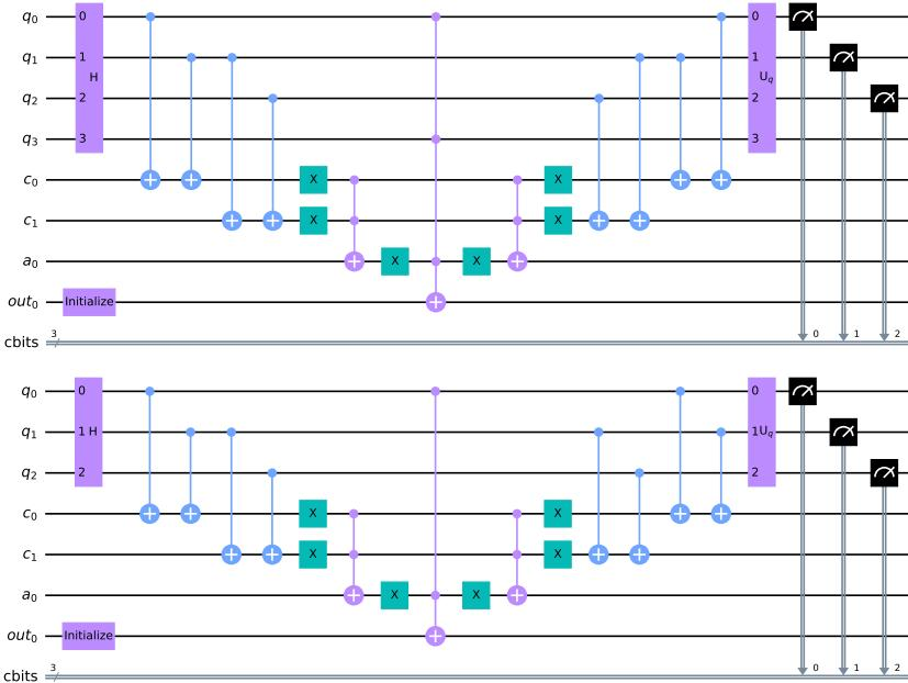
Fig. 2. Quantum circuits, with (top) and without (bottom) an ancillary qubit, used to bootstrap the causal configuration of a three-vertex one-loop Feynman diagram.
