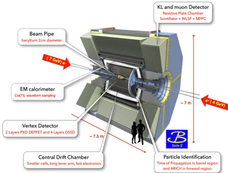
Fig. 1. A schematic diagram of the Belle II detector [7].
