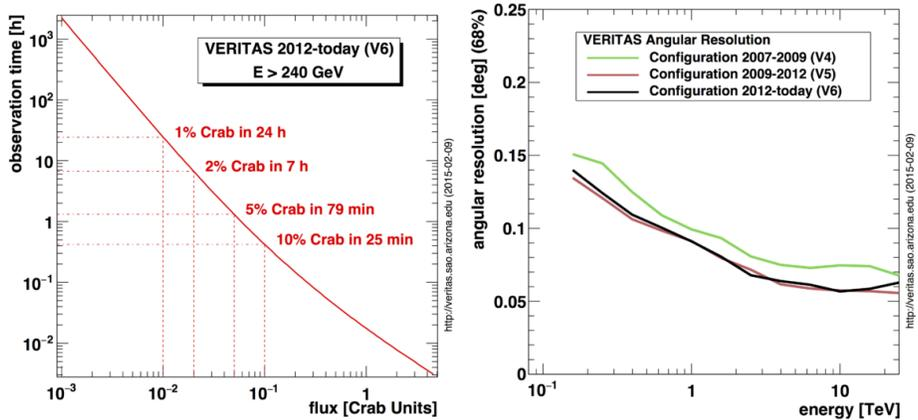
Fig. 1. Left: The VERITAS observation time *versus* source strength to detect a  $5\sigma$  signal. Right: Angular resolution as a function of gamma-ray energy for the VERITAS configuration prior to two major upgrades and for the current configuration. The specifications of the VERITAS gamma-ray instruments are provided at <https://veritas.sao.arizona.edu/>
