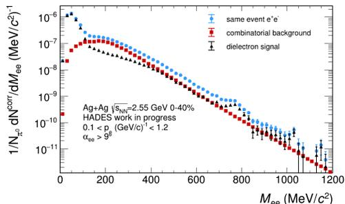
Fig. 1. Efficiency corrected invariant mass spectrum.
