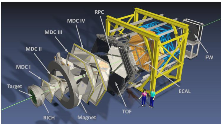
Fig. 1. Schematic expanded view of the HADES detector setup.
