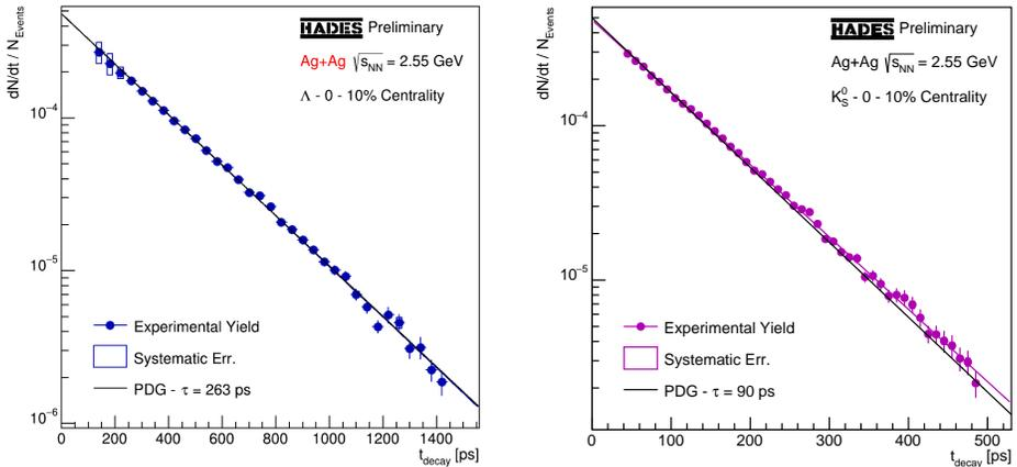
Fig. 3. (Color online) Decay curves of  $\Lambda$  hyperons (left) and  $K_S^0$  mesons (right) from the 0–10% most central Ag(1.58A GeV)+Ag events measured by HADES. The colored lines correspond to the exponential fit functions and the black lines to the PDG literature lifetimes [19].
