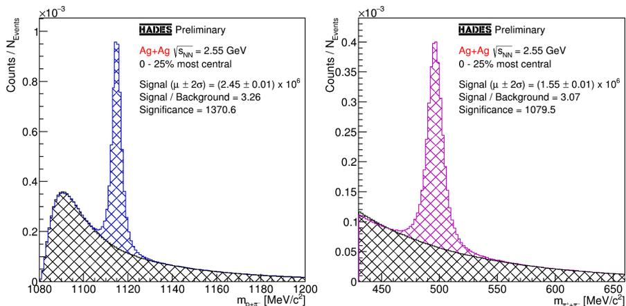
Fig. 2. Invariant mass spectra of  $\Lambda \rightarrow p + \pi^-$  decays (left) and  $K_S^0 \rightarrow \pi^+ + \pi^-$  decays (right) from the 0–25% most central Ag(1.58A GeV)+Ag events measured by HADES.
