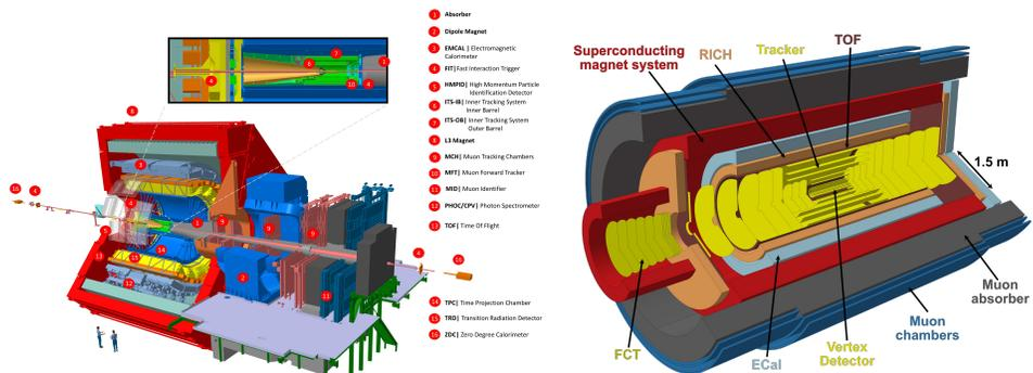
Fig. 4. Detector setup of ALICE 2 in Run 3 (left) and ALICE 3 in Run 5 (right).
