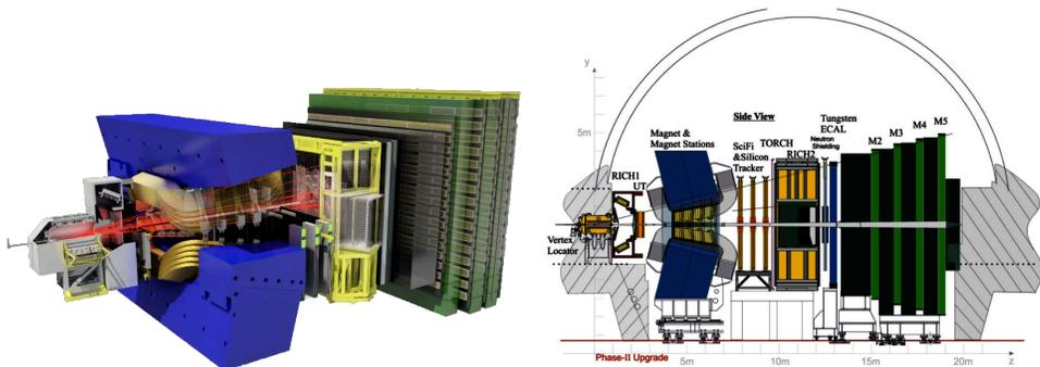
Fig. 3. Experimental setup of LHCb for Run 3 (left) and for Run 5 (right).
