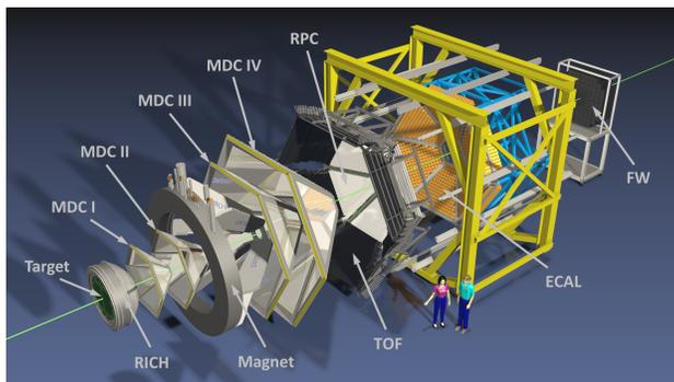
Fig. 1. A 3D scheme of the HADES detector system as used in the March 2019 Ag+Ag data taking, stretched along the beam axis direction for better visibility.
