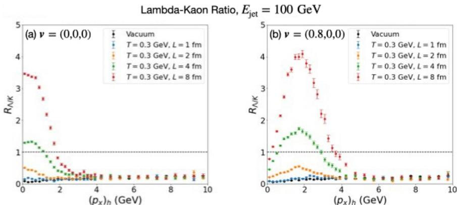
Fig. 5. (Color online) Yield ratios of  $\Lambda$  to  $K$  in jets as a function of momentum in the  $x$ -direction for the brick medium with flow velocity (a)  $\mathbf{v} = (0, 0, 0)$ , and (b)  $\mathbf{v} = (0.8, 0, 0)$ . Each color of the markers represents the path length of the jets in the medium  $L$ .
