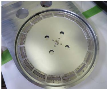
Fig. 8. Photograph of the rotating wheel with sixteen  $^{248}\text{Cm}$  sector targets in the semiclosed inner-target box. The cover plate of the inner-target box is removed to display the interior.
