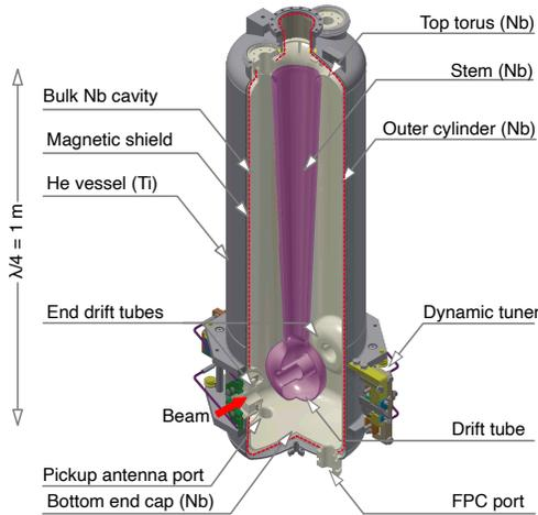
Fig. 4. Schematic view of the SC-QWR for SRILAC.
