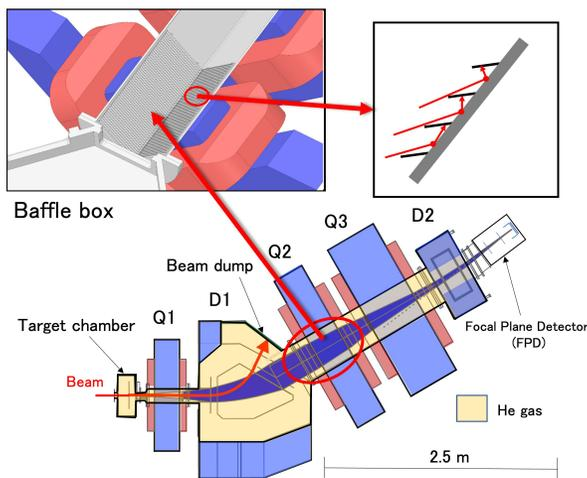
Fig. 5. (Color online) Plan view of GARIS-III. Top left inset: the baffle fin, magnet coil, and iron yoke are indicated in dark gray, reddish-brown, and blue, respectively.
