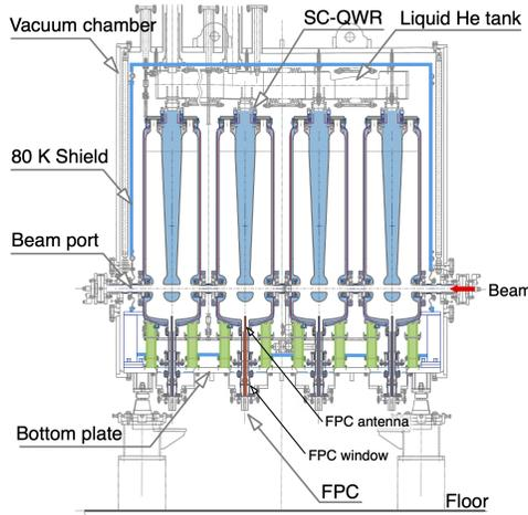
Fig. 3. Side-view of the cryomodule.
