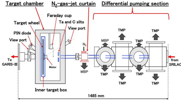
Fig. 6. Layout of the target area.
