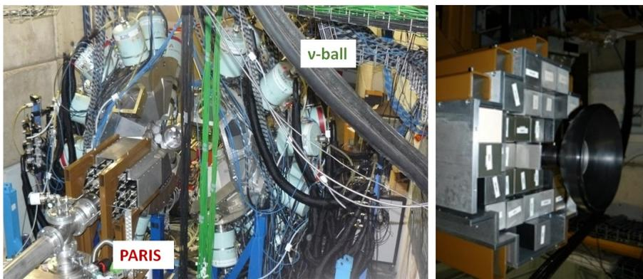
Fig. 2. Photo of the nuBall setup coupled with the PARIS array (left), view of the PARIS array in wall-type geometry used during the campaign (right).
