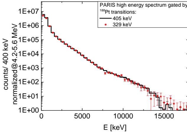
Fig. 4. High-energy gamma-ray measured by PARIS selected by  $^{188}\text{Pt}$  405 keV  $4^+ \rightarrow 2^+$  transition (line) compared to data gated by 329 keV  $14^+ \rightarrow 12^+$  transition (dots).
