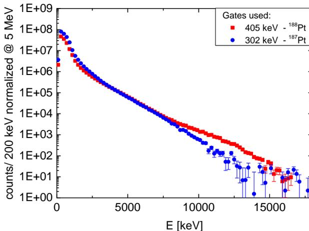
Fig. 3. (Colour on-line) Gamma-ray spectra measured by the PARIS detectors selected by gating on  $^{188}\text{Pt}$  405 keV  $4^+ \rightarrow 2^+$  transition (red squares) and  $^{187}\text{Pt}$  302 keV  $17/2^+ \rightarrow 13/2^+$  transition (blue circles).
