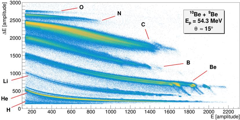
Fig. 1.  $\Delta E$ - $E$  particle identification plot. Nuclei from  $^1\text{H}$  to  $^{16}\text{O}$  are detected. Particles heavier than Be are outside of the optimal gain range which explains the different shapes of the slopes.
