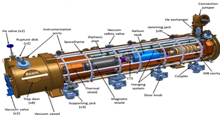
Fig. 7. General assembly view of the ESS cryomodule considered to be adapted for PERLE.
