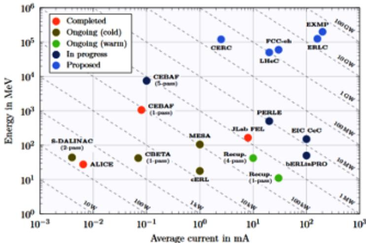
Fig. 1. (Colour on-line) Scatter plot of past (orange), operational (olive green (SC), and green (NC)), planned (dark blue), and potential future (light blue) superconducting ERL facilities on a double logarithmic scale with the maximum beam energy on the vertical and the maximum beam current on the horizontal axis. The dashed diagonal lines indicate the beam power regimes in the scatter plot.
