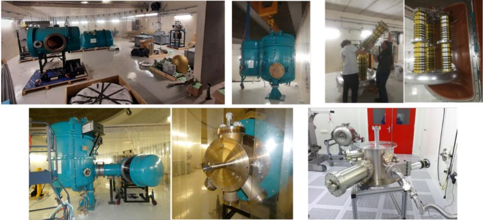
Fig. 5. Sequences of the installation of the photo gun (from top left to bottom right) from March to December 2022. Installation of the high voltage tank with the leak tests; Assembly of the HV columns; tests and modifications to the HV; pre-positioning of the gun; cleaning and test of the anode chamber.
