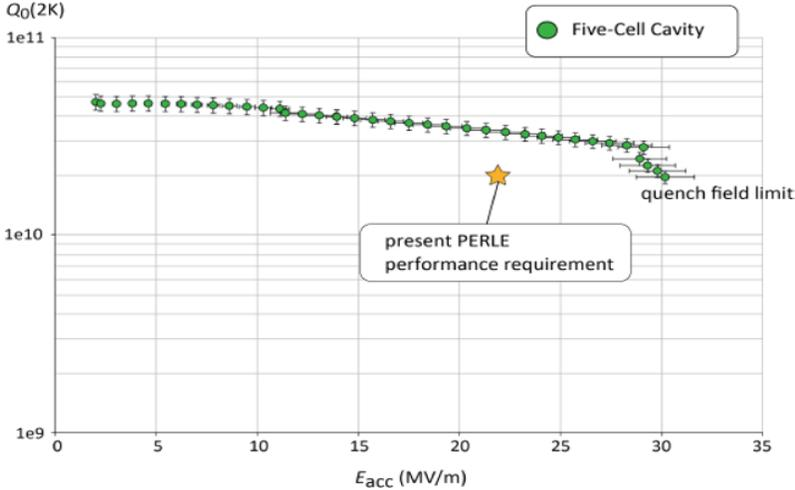
Fig. 6. (Colour on-line) Vertical test result of the 5-cell 801.6 MHz niobium cavity. The star indicates the edge of the performances considered for PERLE operation with a typical CW gradient optimum around 20 MV/m.
