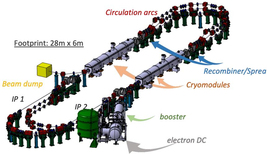
Fig. 2. PERLE layout featuring two parallel linacs, each hosting a cryomodule housing four 5-cell SC cavities, achieving 500 MeV in three passes.
