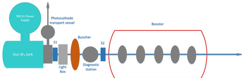
Fig. 4. The layout of the unpolarized injector.
