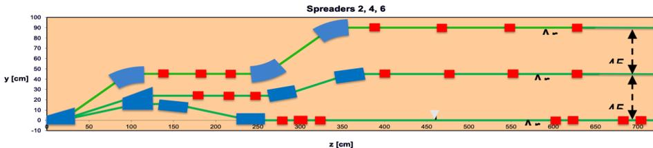
Fig. 3. PERLE spreader design and matching to three circulating arcs.
