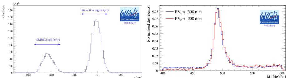
Fig. 3. Left: Distribution of the reconstructed primary vertex longitudinal coordinate for  $pp$  and  $pAr$  collisions. Right: Comparison of the normalised invariant mass distributions for  $K_S^0$  reconstructed with a primary vertex in the SMOG2 ( $PV_z < 300$  mm) or in the  $pp$  ( $PV_z > 300$  mm) region.
