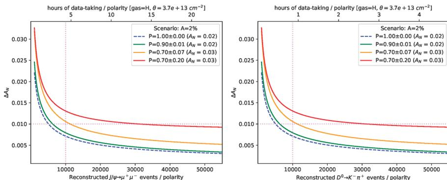
Fig. 9. Number of fully-reconstructed events and data-taking time to reach a given precision on a spin asymmetry at the LHCspin assuming three different polarisation degrees for  $J/\Psi \rightarrow \mu^+\mu^-$  (left) and  $D^0 \rightarrow \pi K$  (right) inclusive production.
