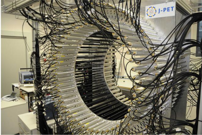
Fig. 1. Image of the first prototype of Jagiellonian Positron Emission Tomograph.
