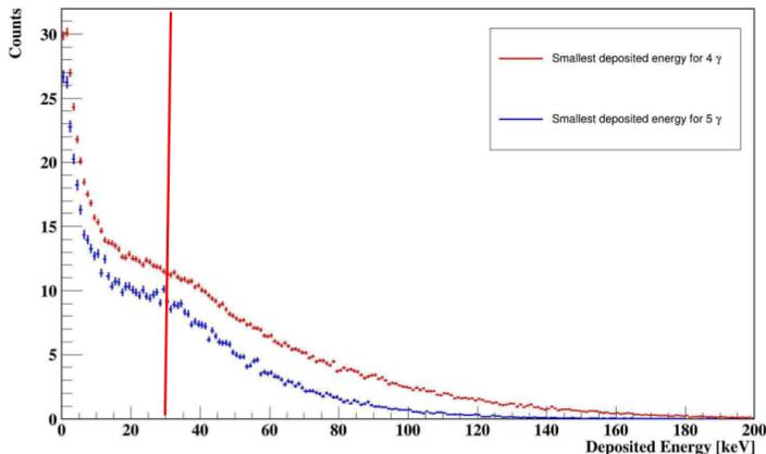
Fig. 3. The smallest energy deposition is shown for  $4\gamma$  and  $5\gamma$  events generated using TGenPhaseSpace. A threshold of 30 keV is applied to limit the electronic noise from the DAQ.
