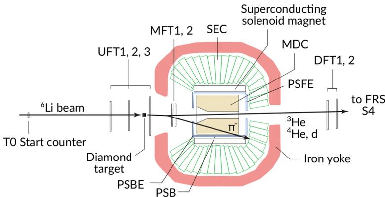
Fig. 1. Scheme of the cylindrical WASA detector apparatus located in the S2 area, which is used to measure light particles such as pions within the solenoid magnet.
