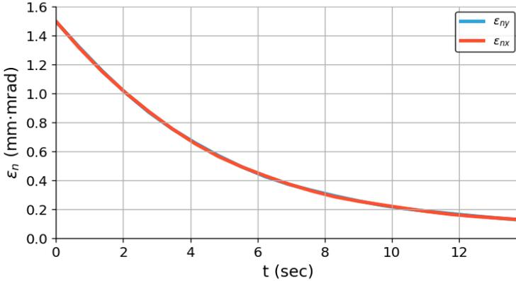
Fig. 3. Simulations of transverse cooling of lithium-like calcium beam. The time-evolution curves of the vertical and horizontal emittances overlap each other — they are precisely equal when the betatron tunes are on the coupling resonance.
