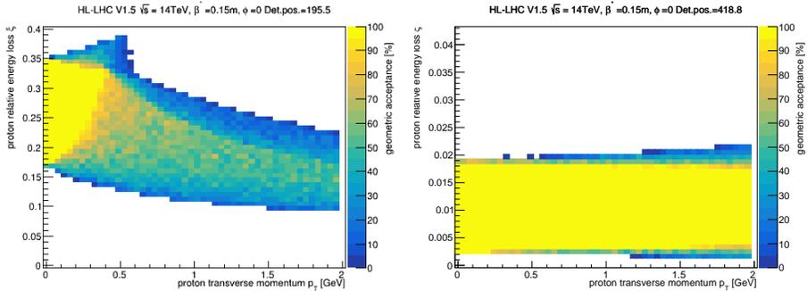
Fig. 2. Geometric acceptance for stations near IP1 and the horizontal crossing angle ( $\phi = 0$ ) for two possible locations: RP1A at 195.5 m (left) and RP4 at 418.8 m (right).
