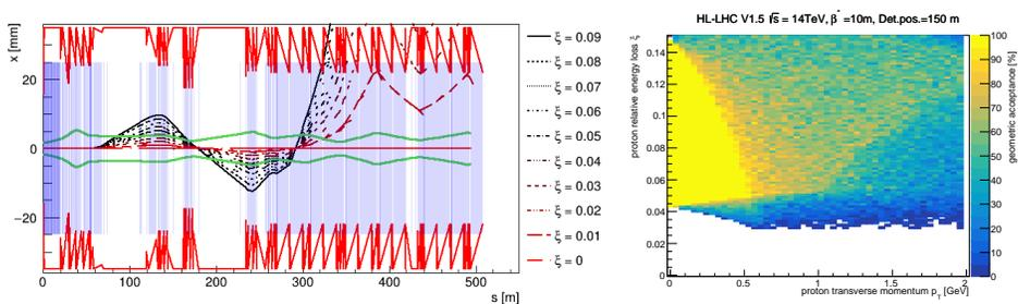
Fig. 4. Left: proton trajectories in the vicinity of the ALICE collision point (IP2). Right: geometric acceptance for pots located at 150 m from IP2.
