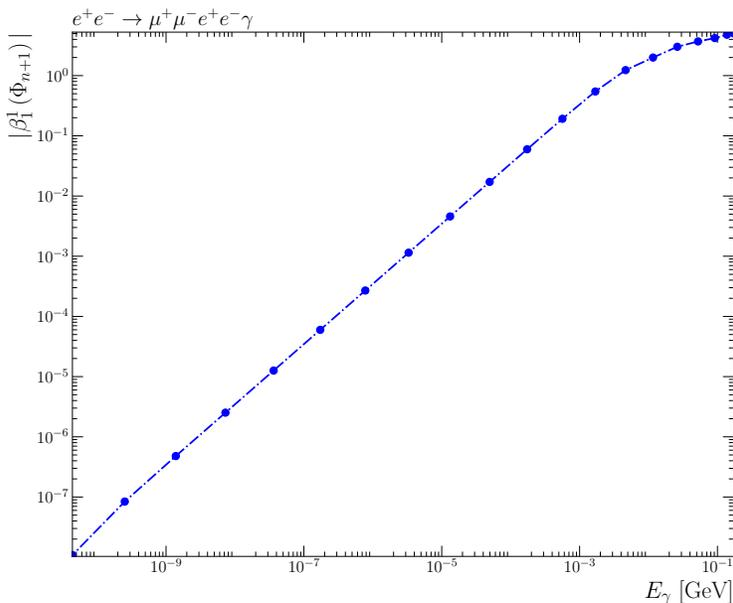
Fig. 3. IR finiteness of the real corrections as the photon approaches the soft limit.
