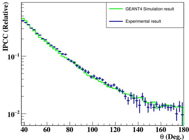
Fig. 4. (Color online) Experimental angular distribution of internal  $e^+e^-$  pairs from the resonant proton capture reaction  ${}^7\text{Li}(p, \gamma){}^8\text{Be}$  (blue/black histogram with error bars) and the angular correlation of the  $e^+e^-$  pairs simulated by Geant4 for the M1 transition of  ${}^8\text{Be}$  with a transition energy of  $E = 17.6$  MeV (green/light gray histogram).
