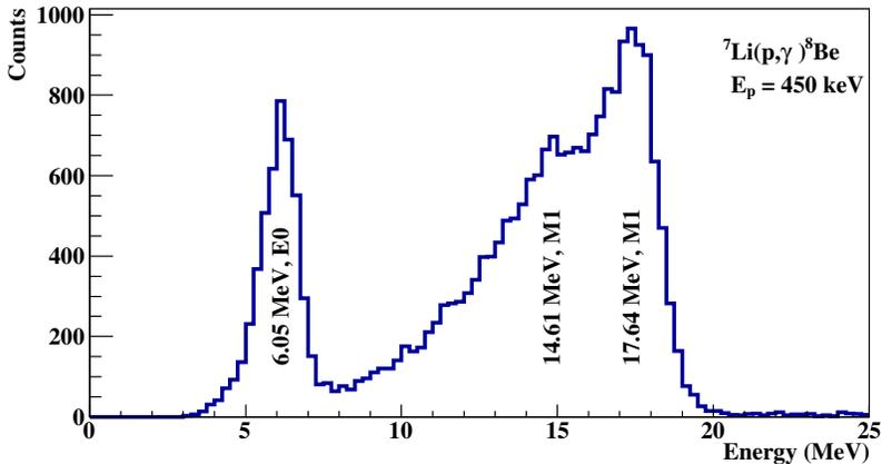
Fig. 2. Energy sum spectrum of the  $e^+e^-$  pairs from the  ${}^7\text{Li}(p,\gamma){}^8\text{Be}$  (M1 transitions) and  ${}^{19}\text{F}(p,\alpha){}^{16}\text{O}$  (E0 transition) reactions. The histogram bin width is 250 keV.
