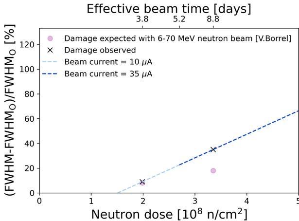
Fig. 1. The evolution of degradation with neutron dose, as observed for the 1332 keV line of  $^{60}\text{Co}$ , is shown. The fits performed are linear, based on only two data points, which describe the behavior of the relative FWHM.
