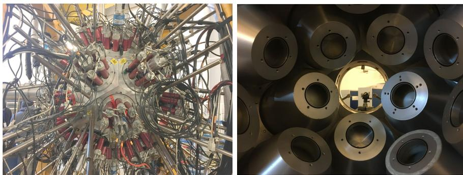
Fig. 1. Global photograph of the LaBr<sub>3</sub> : Ce and CeBr<sub>3</sub> ELIGANT detector array (left panel) [11] mounted in the experimental configuration together with the BGO anti-Compton shield. On the right panel, a front view approximately from the target position is shown.
