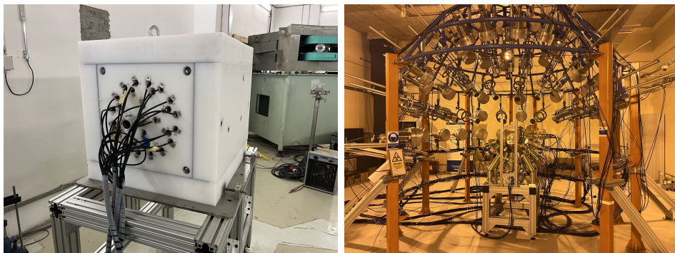
Fig. 1. (Left) Photograph of the ELIGANT-TN neutron counter set up for a preparatory experiment with charged particle beams [19]. (Right) Photograph of the ELIGANT-GN array set up in its \gamma -ray beam experimental area.
