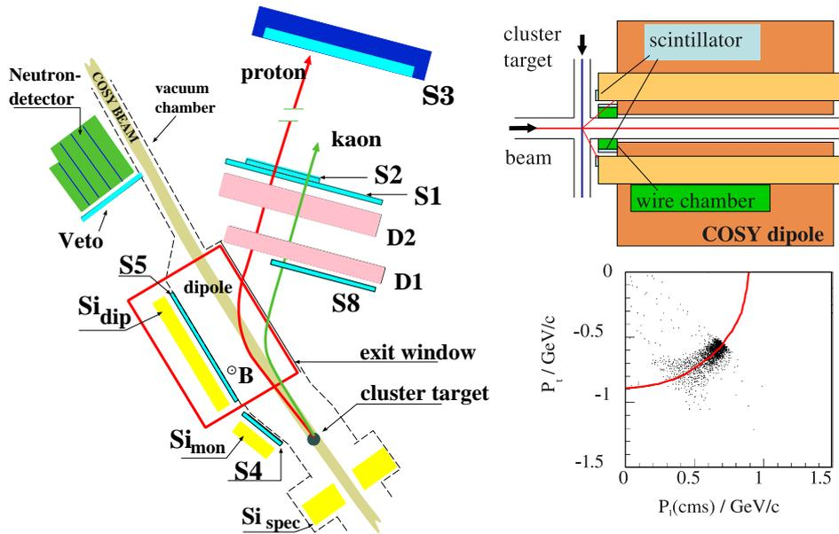
Fig. 2. Sketch of the COSY-11 detection system installed at a COSY machine dipole with drift chambers (D1,D2), scintillators (S1–S8), Si-pad ( $Si_x$ ) and neutron detector (left) and the additional elements (wire chambers and scintillators) to monitor the luminosity (right, upper part). The lower part on the right side shows the well separated elastic events located around the kinematic ellipse.
