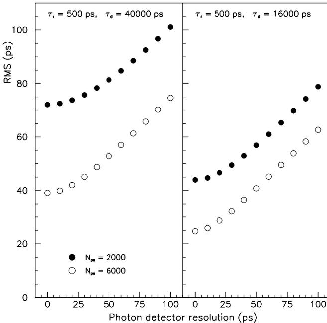
Fig. 3. The scintillator detector timing resolution, calculated with a first photoelectron as a function of photon detector timing resolution (see text for details).
