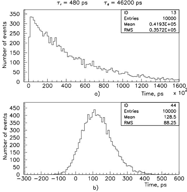
Fig. 2. (a) The timing distribution simulated with bi-exponential timing model, photon detector timing resolution is included,  $\tau_r = 460$ ,  $\tau_d = 46200$ ,  $\tau_{pd} = 125$  ps, FWHM. (b) The distribution of the first PE times from total number of  $N_{PE} = 1932$  PEs in each event. These parameters are equivalent to the experiment [4].
