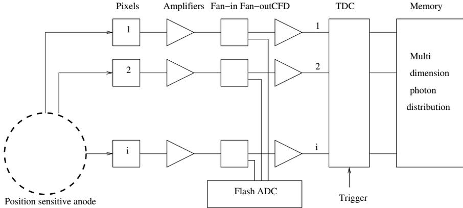
Fig. 1. Schematic of the position sensitive anode and the readout electronics.
