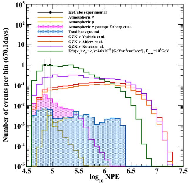
Fig. 3. Brightness measured as number of detected photo electrons (NPE) for the two detected EHE events, including the expected background distribution and several signal models.
