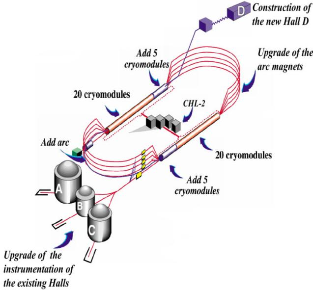
Fig. 2. The JLab accelerator site after the 12 GeV upgrade.
