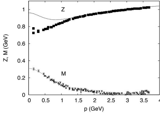
Fig. 4. The quark wavefunction renormalisation,  $Z = 1/A$ , and quark running mass  $M = B/A$ , along with lattice results [4].
