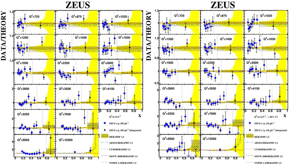
Fig. 2. Ratio of the double-differential cross section in  $x$  and  $Q^2$  and the double differential cross section integrated over  $x$  for NC  $e^-p$  (left) and  $e^+p$  (right) collisions to the expectation from HERAPDF1.5 PDFs as a function of  $x$  at different  $Q^2$  values. For bins with zero measured events, a 68% probability limit is given. For HERAPDF1.5, the uncertainty is given as a band. The predictions of several other PDF sets normalised to HERAPDF1.5 are also shown.
