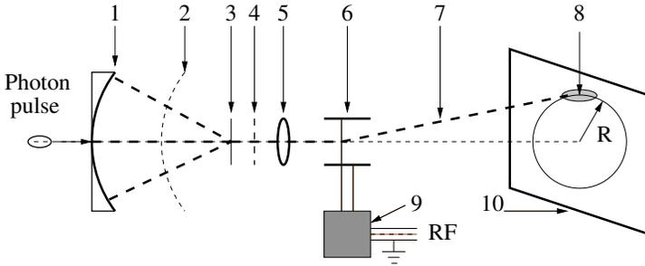
Fig. 3. The schematic layout of the RF phototube with large size photocathode. 1 — photocathode, 2 — electron transparent electrode, 3 — transmission dynode, 4 — accelerating electrode, 5 — electrostatic lens, 6 — RF deflection electrodes, 7 — RF deflected SE, 8 — spot of SE on the PE detector, 9 —  $\lambda/4$  RF coaxial cavity, 10 — PE detector.
