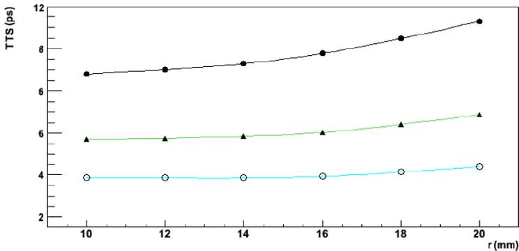
Fig. 4. Simulated TTS of PE at the crossover *vs.* cathode radius for 3 applied accelerating voltages between cathode and accelerating electrode in a “spherical-capacitor” region. Filled circle 2.5 kV, triangle 5.0 kV, open circle 10 kV.
