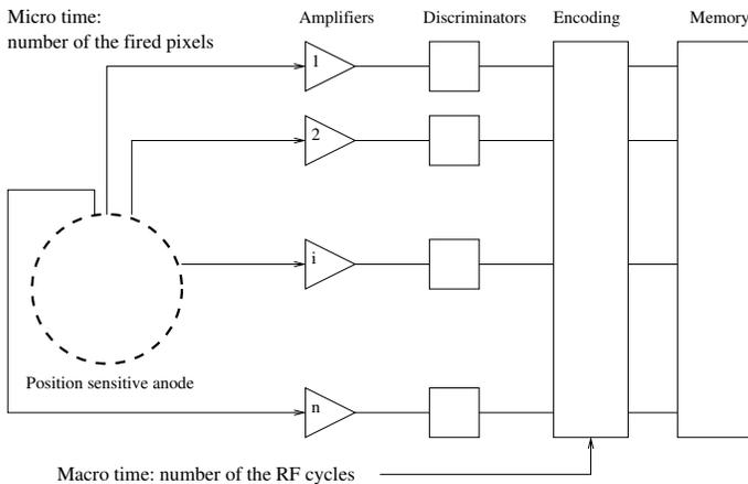
Fig. 6. Schematic of a timing system based on the pixelated anode RF PMT.
