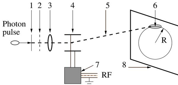
Fig. 1. Schematic diagram of a small area photocathode RF PMT: 1 — photocathode, 2 — electron transparent anode, 3 — electrostatic lens, 4 — electrodes of the RF deflector, 5 — RF deflected PE, 6 — spot of PE on the PE detector, 7 —  $\lambda/4$  coaxial RF cavity, 8 — PE detector.
