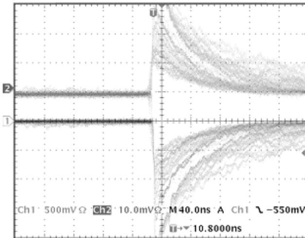
Fig. 5. Nanosecond signals directly from APD (top) and after preamplifier (bottom).
