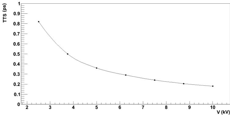
Fig. 2. Simulated TTS *vs.* applied accelerating voltage.
