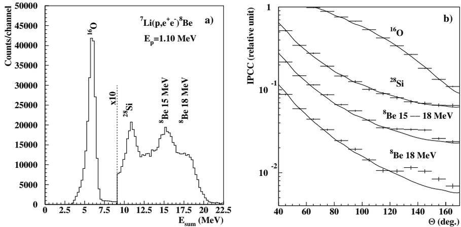
Fig. 1. Measured total energy spectrum (a) and angular correlations (b) of the  $e^+e^-$  pairs created in the different transitions labelled in the figure, compared with the simulated angular correlations assuming E0 (from the  ${}^{16}\text{O}$  peak) and M1+E1 mixed transitions from the other peaks.
