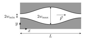
Fig. 1. Schematic representation of a single cell of a channel with the periodicity L, bottleneck half-width  $w_{\min}$  and maximal half-width  $w_{\max}$ . The shape of the structure is defined by Eq. (2). The constant, applied bias F is acting only along the length of the channel.
