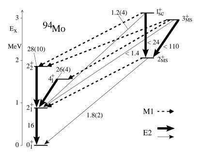
Fig. 1. Partial level scheme of  ${}^{94}$ Mo (from [13]). The numbers denote B(E2) values in Weisskopf units. For B(M1) values see Table I.
