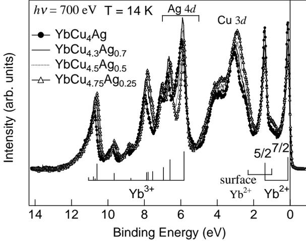
Fig. 1. Valence-band spectra of  $\text{YbCu}_{5-x}\text{Ag}_x$  ( $x = 1.0, 0.7, 0.5, 0.25$ ). The photon energy is 700 eV. Background due to inelastically scattered electrons has been subtracted from each spectrum. The bar diagrams are from the multiplet calculation in Ref. [9].
