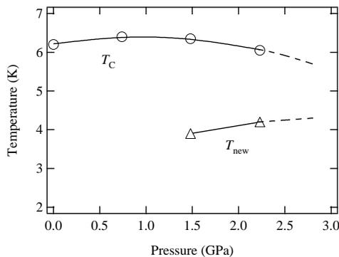
Fig. 3. Pressure dependence of the Curie temperature and new anomalies of the  $\text{CeCu}_9\text{Sn}_4$ .
