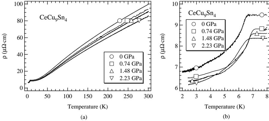
Fig. 2. (a) Temperature dependence of the electrical resistivity of the  $\text{CeCu}_9\text{Sn}_4$  at various pressure. (b) Low temperature part of the temperature dependence of the electrical resistivity of the  $\text{CeCu}_9\text{Sn}_4$  at various pressure.
