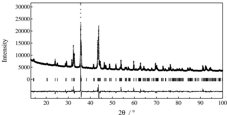
Fig. 1. X ray diffraction pattern using  $\text{Cu K}\alpha$  of  $\text{CeCu}_9\text{Sn}_4$  (cross symbols) and calculated pattern by using of Rietveld method [4] (solid line). Lower solid line is the residual curve.
